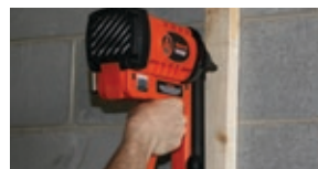
Furring attachment—perfect fastening every time in soft and hard base materials
